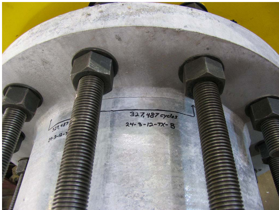
Figure 5.4: Typical Failure of Texas full penetration weld connection
