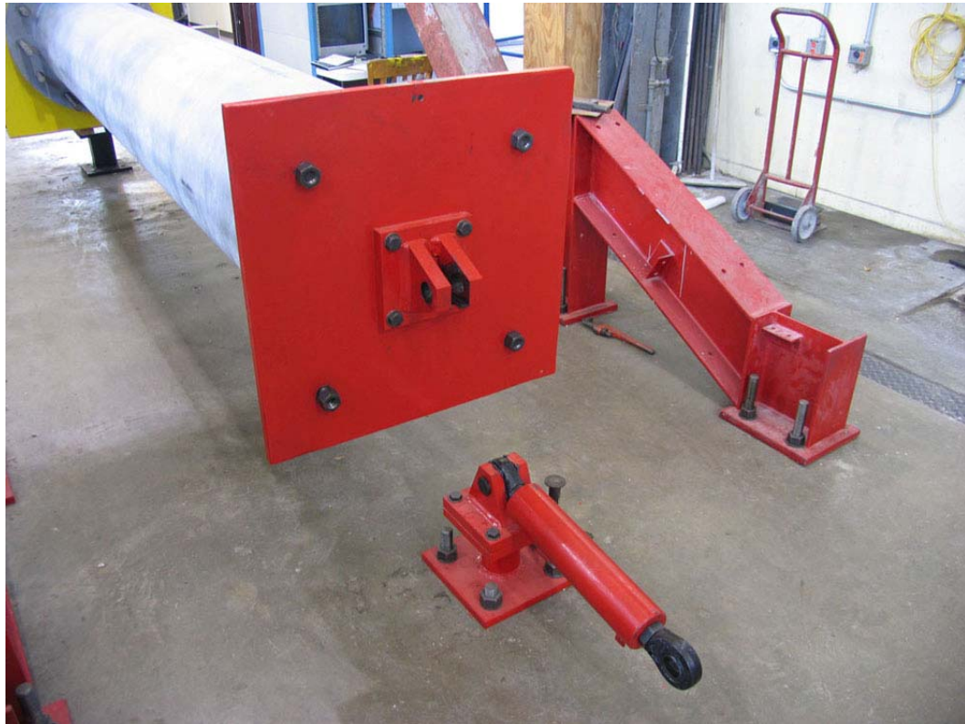
Figure 4.1: Pole specimens released from reaction supports
