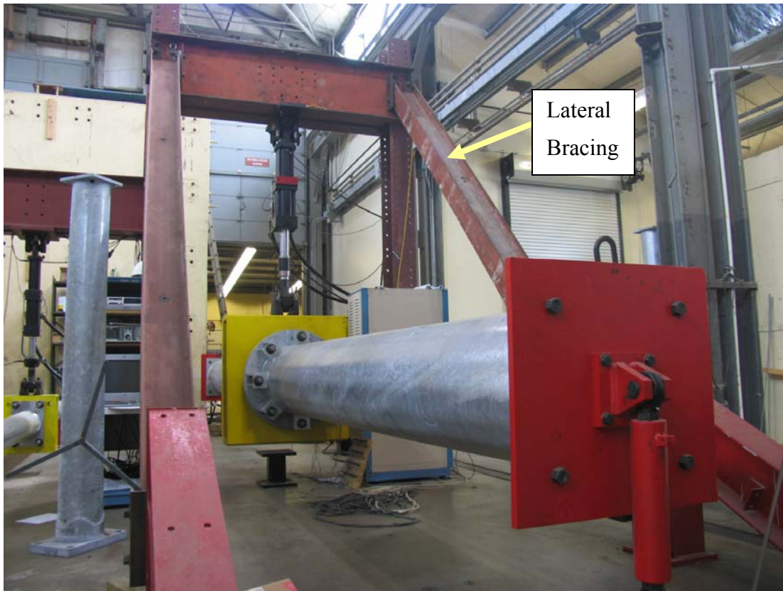
Figure 3.9: Portal loading frame showing lateral bracing
