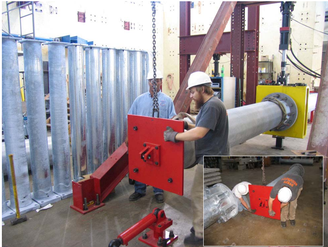
Figure 4.2: Transfer of reaction plates to new specimens
