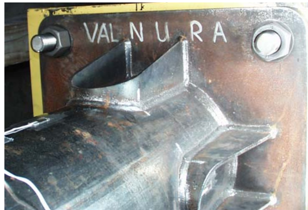
Figure 2.8: U-Rib stiffened horizontal mast-arm
